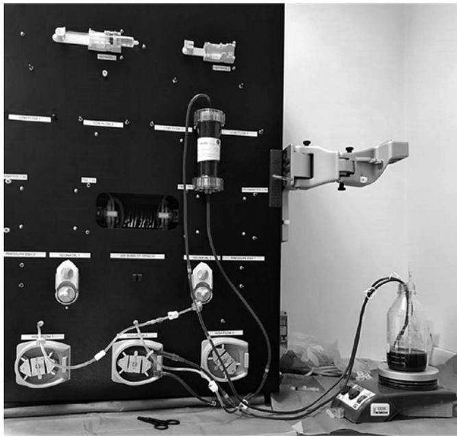
**Fig. 2.** Experimental set-up of the dedicated testing platform, GALILEO machine, used to acquire pressure pre and post cartridges at different blood flow rates.
