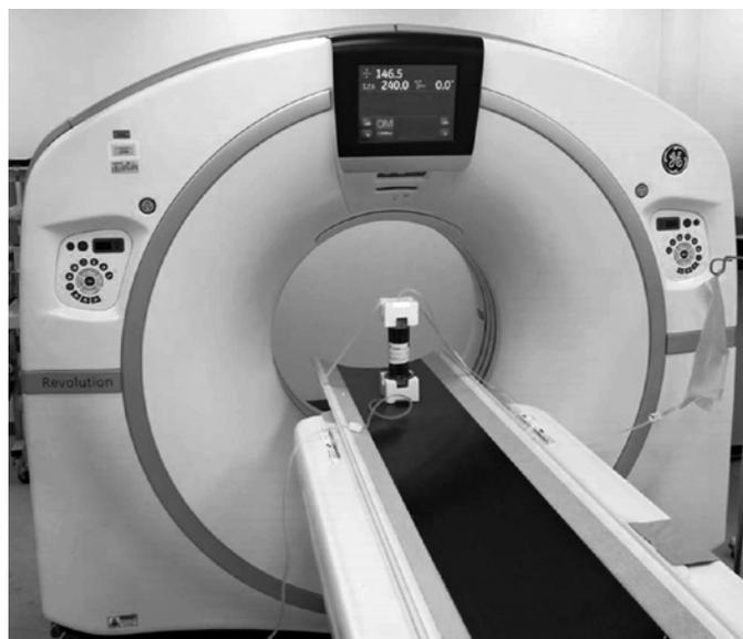
**Fig. 1.** Experimental set-up for CT imaging acquisition. The cartridge was held in vertical position by a support and placed in the middle of the gantry. Flow is direct from the bottom to the top.
