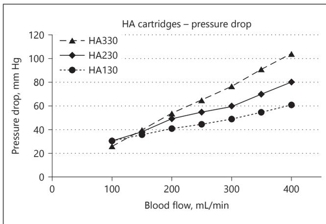
**Fig. 6.** Pressure drop of the 3 cartridges at different blood flow rates.
