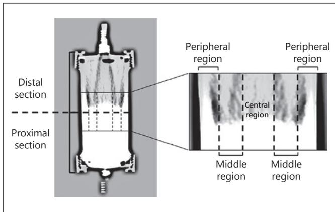
**Fig. 5.** Representative frame of progression profile in the distal section of cartridge HA230. Higher velocity profiles are observed in central and peripheral regions of the cartridge, while in the middle regions velocity is lower.
