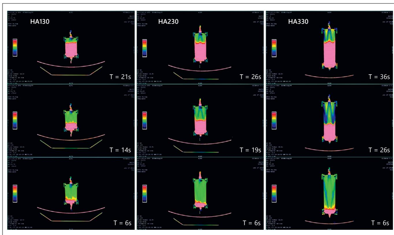
**Fig. 3.** Flow distribution in the 3 cartridges – HA130, HA230, HA330. From the bottom to the top, the frames show the dye progression inside the devices.
